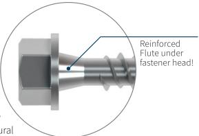
**C1022 steel** coil used in the manufacture of the roofglory fastener is a low-carbon steel, ideal for fastener use due to its greater strength characteristics, good ductility and machinability for quality fastener fabrication, and noted for its benefit in structural applications. Maximum carbon content is 0.23%.
